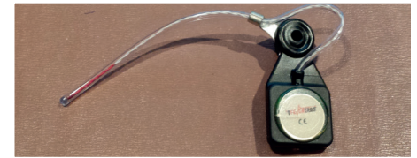
A device which sits in the ear for monitoring fever in calves
